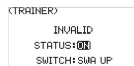
3. Set a switch. In the menu, select a switch and its corresponding position to finish, or you can toggle the corresponding physical switch on the transmitter to finish.
