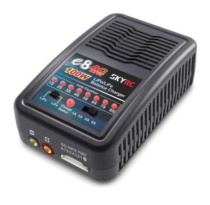
SKYRC e8 Charger is an economic, high quality 100-240V AC balance charger, designed for charging LiPo and LiFe batteries from 2-8 cells in balance mode. The circuit power is 100W and max charge current can reach to 6A. There are four kinds of charge current 1A/3A/5A/6A that can be selected. You could select the proper charge current according to the battery capacity.
