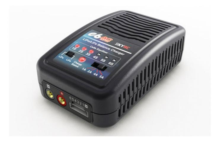
SKYRC e6 Charger is an economic, high quality 100-240V AC balance charger, designed for charging LiPo and LiFe batteries from 2-6 cells in balance mode. The circuit power is 50W and max charge current can reach to 5A. There are four kinds of charge current 1A/2A/4A/5A that can be selected. You could select the proper charge current according to the battery capacity.
