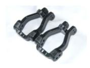
With these 6° Caster Blocks you can reduce the caster even more. In combination with the Kick-Up of the Chassis and the Hing-Ping holders you can go down to 12°.
