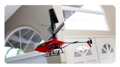
The incredible stability and durability of the Ares Chronos CX 75 makes it easy and fun for anyone to fly an RC helicopter. The co-axial, counter-rotating blade design offers unsurpassed stability that will have any pilot hovering like a pro in no time, while fully proportional controls deliver excellent maneuverability and control.
