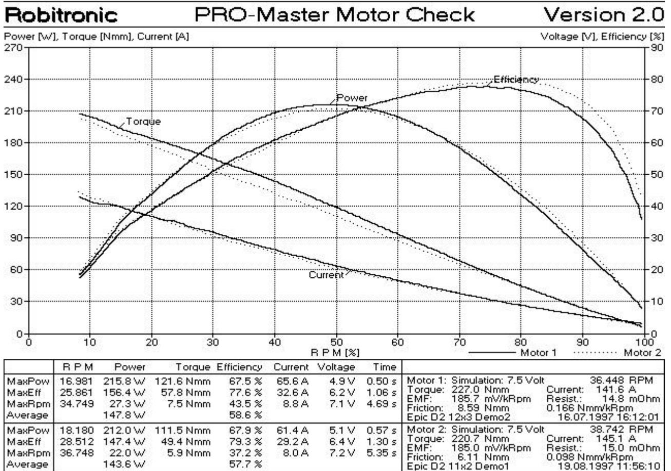
The benchmark data are displayed as dotted lines. In the table the benchmark data are displayed in the lower table (Motor 2).
