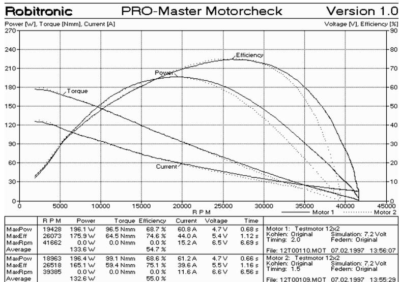
The motor timing is advanced by one step.
