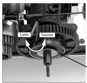
Note: Outer (1st) Spur gear removed for photo.
