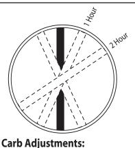
Make all carburetor adjustments in one hour increments. Imagine the slot in the needle is the hour hand on a clock. Adjust it as though you were moving the hour hand from one hour to the next or previous one.
