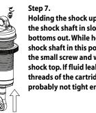
Holding the shock upright, push the shock shaft in slowly until it bottoms out. While holding the shock shaft in this position, replace the small screw and washer in the shock top. If fluid leaks around the threads of the cartridge, it is probably not tight enough.
