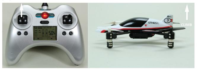
Decreasing the speed of the propellers/rotor blades by lowering the left-hand stick will cause the model to descend.
