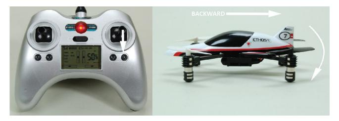
The elevator trim can be used to help keep the quadcopter from drifting forward or backward when hovering and with no right-hand stick input. For example, if the quadcopter drifts forward when hovering add backward (up) elevator trim by pressing the right-hand elevator trim button (the right side of the rocker switch) located on the top right 'corner' of the transmitter until the quadcopter hovers as level as possible with no forward drifting.
