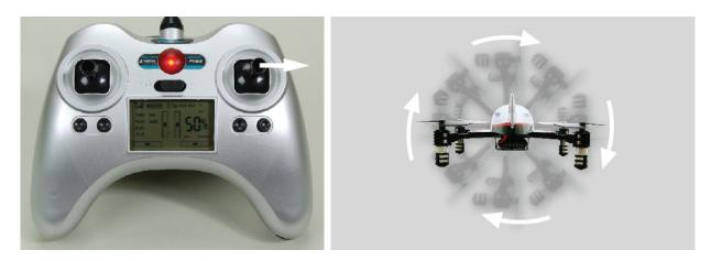
After the 360 degree flip is complete the transmitter will automatically deactivate AFM and the audible beeps/tones will stop (indicating AFM is no longer active). You can continue to fly 'normally' until you're ready to perform your next flip by pressing the AFM button again.
