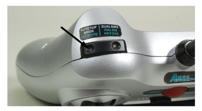
The Automatic Flip Mode (AFM) is activated by pressing the 'AUTO FLIP MODE' button (the left side of the rocker switch) located on the top left 'corner' of the transmitter. You will feel a 'click' and also hear continuous audible beeps/tones that indicate you've activated AFM after pressing the button. At the same time the LED indicator on the 4-in-1 control unit will switch from glowing solid green to glowing solid red.
