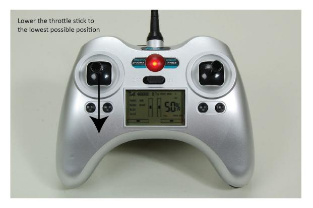
Power the transmitter on and confirm that the LED indicator is blinking red. Then, slide the flight battery into the battery mount (located on the bottom of the main frame) and connect it to the control unit.
