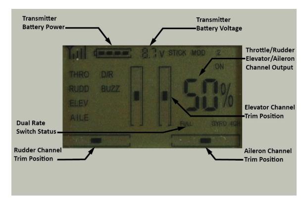
The unique LCD screen displays a variety of data when the transmitter is powered on:
