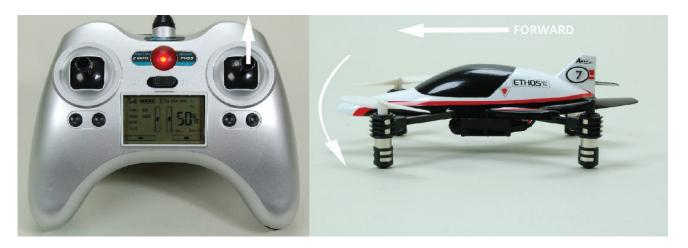
Pulling the stick backward will pitch the tail the quadcopter downward, allowing it to be flown backward.
