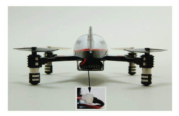
When the battery is connected securely carefully 'tuck' the wire leads and connectors into the body/canopy of the quadcopter. YOU MUST ENSURE THE WIRE LEADS AND CONNECTORS WILL NOT COME INTO CONTACT WITH THE PROPELLERS/ROTOR BLADES WHEN THEY SPIN.
