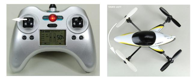
Moving the stick to the right will turn (yaw) the nose of the quadcopter to the right about the vertical axis. This is accomplished by increasing the speed of the right-front and left-rear propellers/rotor blades while decreasing the speed of the left-front and right-rear propellers/rotor blades.
