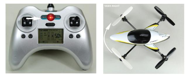
The rudder trim is used to help keep the nose of the quadcopter from turning (yawing) to the left or right when 'hovering' and without any rudder/left-hand stick input. For example, if the nose of the quadcopter turns to the right when hovering add left rudder trim by pressing the left-hand rudder trim button until the nose of the quadcopter stays as close to straight as possible with no further input.
