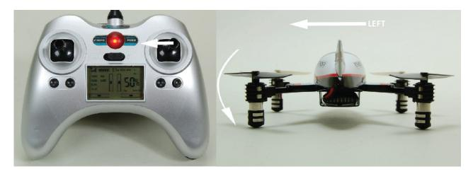
Moving the stick to the right will roll the quadcopter to the right, allowing it to be flown to the right.
