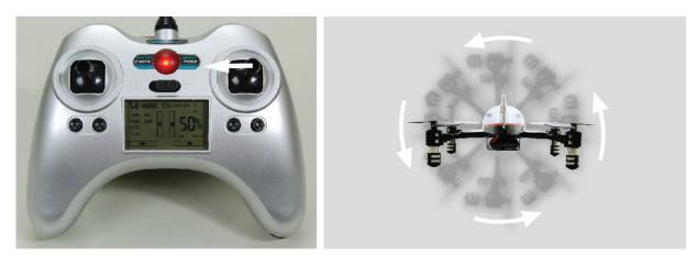
Moving the right-hand/aileron stick all the way to the right will cause the quadcopter to automatically flip a full 360 degrees to the right from the starting position.
