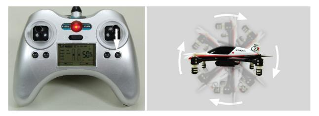
Moving the right-hand/aileron stick all the way to the left will cause the quadcopter to automatically flip a full 360 degrees to the left from the starting position.
