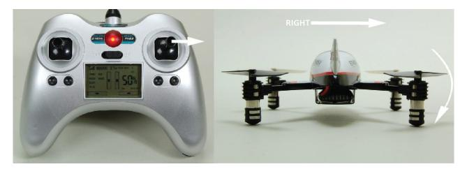
The aileron trim can be used to help keep the quadcopter from drifting left or right when hovering and with no right-hand stick input. For example, if the quadcopter drifts to the right when hovering add left aileron trim by pressing the left-hand aileron trim button until the quadcopter hovers as level as possible with no drifting to the right.
