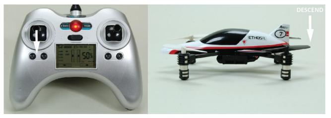
After lifting the model off the ground you can 'hover' by carefully moving the left-hand stick up and down slightly as needed so the model will maintain altitude without climbing or descending. Moving the left-hand stick to the left will turn (yaw) the nose of the quadcopter to the left about the vertical axis. This is accomplished by increasing the speed of the left-front and right-rear propellers/rotor blades while decreasing the speed of the right-front and left-rear propellers/rotor blades.
