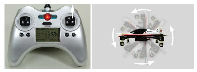
Pulling the right-hand/elevator stick backward to the lowest possible position will cause the quadcopter to automatically flip a full 360 degrees backward from the starting position.
