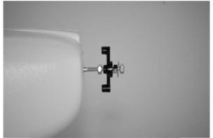
Measure to be sure no more than approximately 3/32" (2.5mm) of the shaft extends beyond the front hex nut. Otherwise adjust the position of all parts accordingly to ensure the prop saver works correctly.
