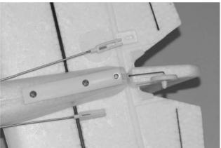
When engaged properly the tail mount should fit almost flush against the fuselage. Now you can slide the two 'button' (small) head screws into the recessed openings in the mount and tighten them securely. Be careful when tightening these screws because tightening them too much can strip/break the plastic posts and/or damage the tails/fuselage.
