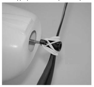
**OPTIONAL:** For improved appearance and protection of the gearbox propeller shaft you can cut down/shorten the shaft accordingly. However, note that if you shorten the shaft it will not be possible to switch to standard installation of the propeller and spinner without changing to a new gearbox propeller shaft (AZS1212) first.
