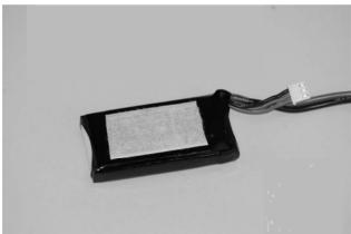
Before installing the battery in the airplane you'll need to connect it to the ESC (Electronic Speed Control). YOU MUST BE CAREFUL TO ENSURE PROPER POLARITY BEFORE CONNECTING THE BATTERY TO THE ESC. By orienting/aligning the wire leads of the battery and ESC so they're 'red to red' and 'black to black' you'll be able to make the connection with correct polarity.
