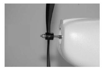
IMPORTANT NOTE: Before installing the spinner it will be helpful to turn on the transmitter, connect the LiPo battery arm the ESC (as outlined earlier in this section) then carefully run the motor and ensure the propeller tips are 'tracking'
