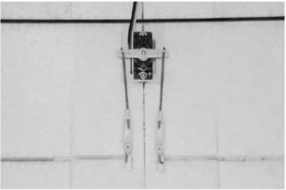
After installing the servo arm on the output shaft in the position with the best possible alignment use one of the suitable screws included with the servo to secure the servo arm to the output shaft (do not over-tighten!).
