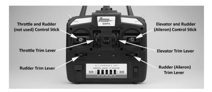
IMPORTANT NOTE: As is typical of most '3-channel' models that are equipped with a rudder for primary 'turning' control, the 'aileron' control stick/channel is used to control the rudder on the Gamma 370. This helps to ensure an easier transition to controlling '4-channel' models equipped with ailerons later on.
