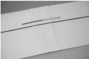
After assembling the two wing panels locate the plastic 'wing cover'. This cover helps protect the wing from the rubber bands used to attach it to the fuselage while also providing additional support for the wing joint.
