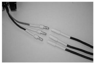
It's easier to check and properly set the direction of rotation for the brushless motor BEFORE installing it and the brushless ESC. To check, start by connecting the three gold 'bullet' connectors from the motor leads to the mating connectors on the wire leads of the ESC. You can connect the leads/connectors in any order then temporarily plug the white/red/black 3-wire lead from the ESC into the 'THRO' (throttle) channel of the receiver.
