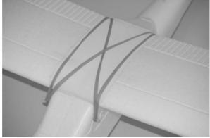
For first-time and low-time pilots that will not be performing aerobatics we recommend installing only these four (4) rubber bands total. This offers plenty of security for the wing while also allowing it to shift a bit more easily on the fuselage. However, for experienced pilots that will be performing aerobatics we recommend installing an additional two (2) rubber bands (for a total of six [6]) that 'cross' just like the first and second ones did.
