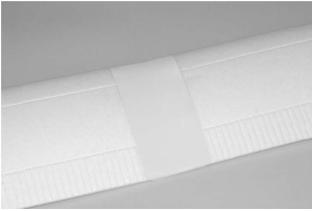
NOTE: In some cases it may not be possible for all edges of the cover to fit flush against the surface of the wing. This is not typically a problem as the rubber bands used to attach the wing to the fuselage will help hold the edges of the cover in place. However, depending on the fit of some parts and the environmental conditions it may be helpful to apply transparent 'packing' tape and/or Cyanoacrylate (CA) glue (we recommend Medium/Gap-Filling or Thick CA) to better secure the edges.
