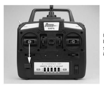
Decreasing the speed/RPM of the propeller by lowering the left-hand stick will decrease the speed of the model and reduce thrust making it possible to descend/decrease altitude.
