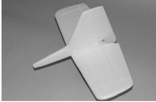
Next, carefully slide the forward section of the vertical tail into the corresponding area on the fuselage then 'lower' the tail section into place on the fuselage so the small 'tabs' on the bottom of the horizontal tail align and fit into the recesses in the fuselage. Now the entire tail section should be 'press-fit' to the fuselage.
