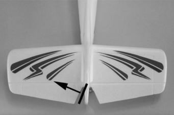
Moving the stick to the right will move the rudder to the right. This will roll/turn the airplane to the right.
