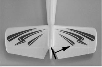
The rudder (aileron) trim lever (located immediately below the right-hand stick) can be used to help keep the airplane from drifting/turning left or right during flight with no right-hand stick/rudder input. For example, if the airplane drifts to the right in flight, add left trim until the airplane flies as straight as possible without drifting.
