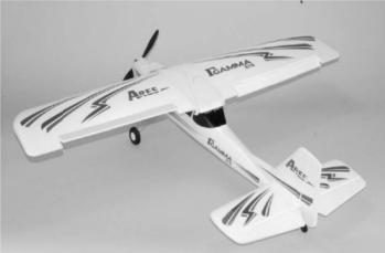
Moving the stick to the right will move the right aileron up and the left aileron down. This will roll/turn the airplane to the right.
