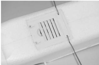
To remove the LiPo flight battery first remove the hatch cover and pull the wire leads and connectors out of the battery compartment. Then, carefully pull the battery out of the compartment by separating the hook-and-loop material mounted inside the fuselage and on the battery. Disconnect the battery from the ESC and DO NOT power off the transmitter until the LiPo flight battery is removed from the airplane and disconnected from the ESC.
