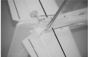
After connecting the clevises to the control horns view the vertical tail and rudder from directly above. The rudder should be 'in line' with the vertical tail when it's properly 'centered'. However, if the rudder is angled off to the right or left you can adjust the length/position of the pushrod/clevis so the surface is centered 'mechanically' while the rudder channel trim is centered.
