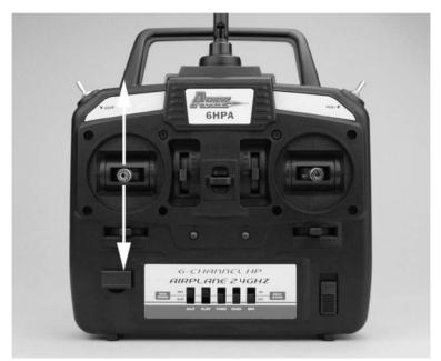
Moving the stick upward will increase the speed/RPM of the propeller. Increasing the speed of the propeller increases the speed of the model and also provides the thrust needed to climb/increase altitude.
