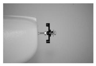
Measure to be sure no more than approximately 3/32" (2.5mm) of the shaft extends beyond the front hex nut. Otherwise adjust the position of all parts as needed so no more than approximately 3/32" (2.5mm) of the shaft extends beyond the nut. **This is critical to ensuring the prop saver works correctly!**
