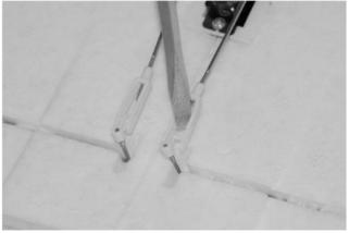
After connecting the clevises to the control horns/brackets view the trailing (rear) edge of the ailerons and wing from directly behind. The trailing edges of the ailerons should be 'in line' with the trailing edges of the wing when ailerons are properly 'centered'. However, if the ailerons are 'off center' you can adjust the length/position of the pushrods/clevises as needed.
