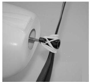
To install the propeller rotate it as necessary until it lines up with, slides over and fully 'engages' the front hex nut in a position as close to perpendicular (when viewed from the front) to the prop saver as possible. Then use a small rubber band to attach the propeller to the prop saver. Be sure to wrap the rubber band around the propeller and prop saver enough times to keep the propeller as secure as possible (while still allowing for some limited flexibility)
