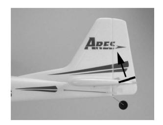
The elevator trim lever (typically located immediately to the left of the right-hand stick) can be used to help keep the airplane from climbing or descending when in 'cruise flight' and with no right-hand stick/elevator input. For example, if the airplane climbs when attempting to cruise and maintain a given altitude, add down elevator trim by sliding the trim lever upward until the airplane flies as level as possible and maintains the desired altitude at cruise speed.
