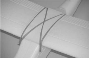
For pilots that will not be performing advanced aerobatics we recommend installing only these four (4) rubber bands total. This offers plenty of security for the wing while also allowing it to shift a bit more easily in the unfortunate event of a crash or less than perfect takeoff or landing. However, for pilots that will be performing advanced aerobatics we recommend installing an additional two (2) rubber bands (for a total of six [6]) that 'cross' just like the first and second ones did.
