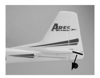
Pulling the stick backward/downward will raise the elevator and pitch the nose of the airplane upward to climb.
