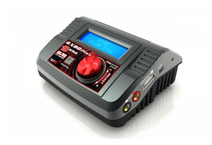
SkyRC 6x80 Plus is a high-performance, micro processor control charge/discharge station with battery management suitable for use with all current battery types. With integral equalizer for six-cell, Lithium- Polymer (LiPo), Lithium-Ferrum (LiFe) and Lithium-Ion (LiIon) batteries. Maximum 10A charge current; maximum 80W charge power; can be powered by a 12 Volt car battery or from 100V-240V via the built in switch-mode power supply.
