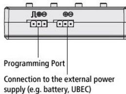
**Warning!** The battery must be disconnected from the ESC before connecting the ESC to the programming box. Otherwise, your ESC cannot be "connected" to the programming box.
