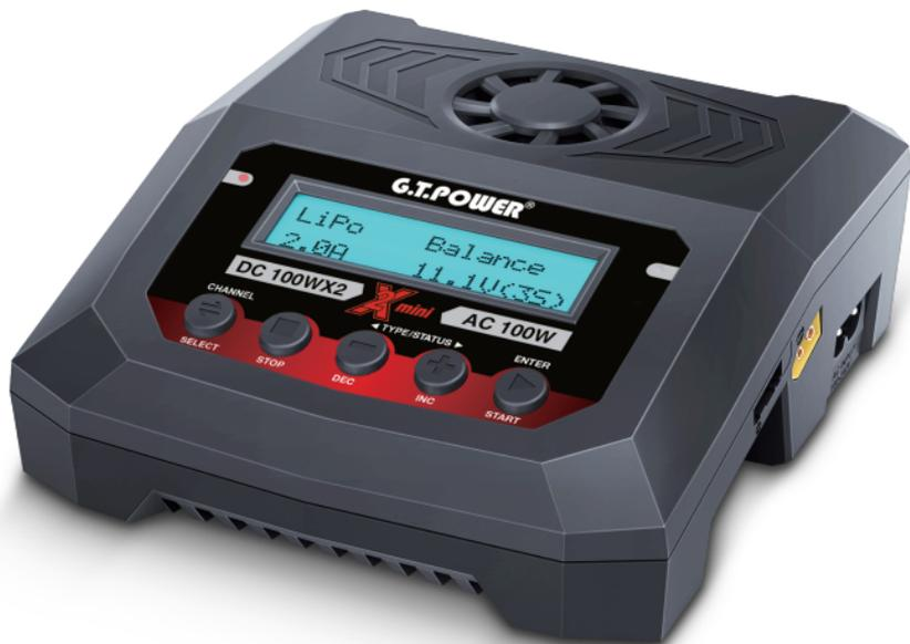
Thanks for purchasing GT Power X2mini Charger. This is a charger with built in microprocessor and newest program. This charger can support 2 channels charging, can charge 2 different battery types at the same time. This charger with fashion design, easy to operate. Please read the manual completely and carefully before using.
